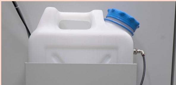
Water supply tank
