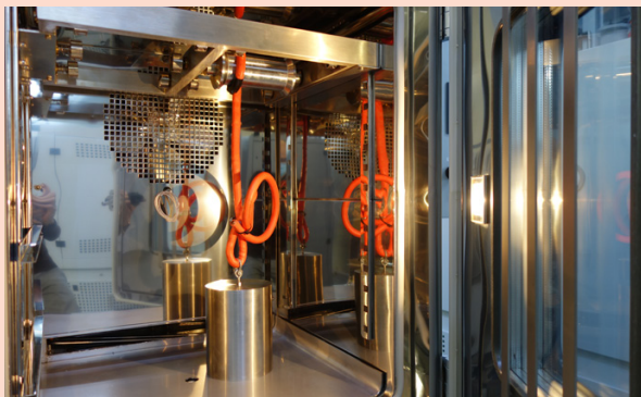
Cold Bend Cables Testing
